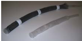
Previous worm robot with 10 cm long McKibben style actuators
