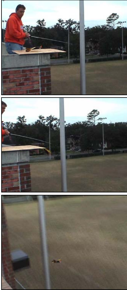
Fig. 8: a) MMALV nears the edge of the structure; b) MMALV walks off of the building, entering a “power dive”; c) lift is produced, and the vehicle pulls out of the dive
