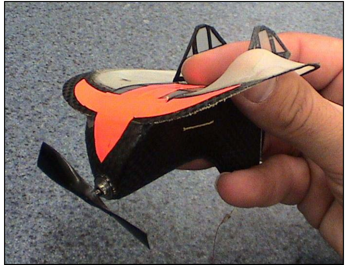
Fig. 2: Demonstrating the flexibility of the wing on the UF-MAV
