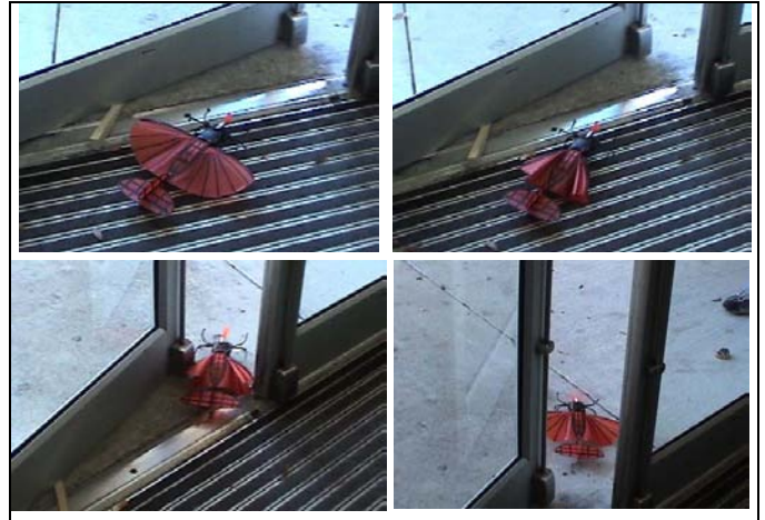
Fig. 9: When (a) MMALV is confronted with a narrow passage, it (b) retracts its wings, (c) negotiates the passage, and (d) redeployes its wings.
