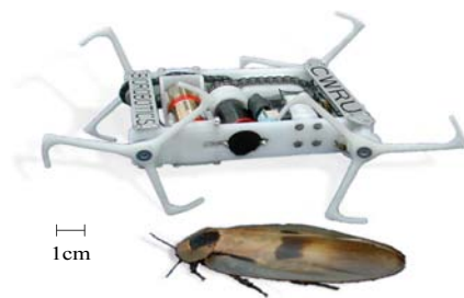
Fig. 3: Relative sizes of Mini-Whegs™ and Blaberus giganticus cockroach
