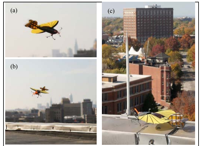
Fig. 1: In the proposed mission, MMALV must (a) fly up to 1.5km from the launch point to the target zone, (b) land on a rooftop within the target zone, and (c) walk to the edge of the building to survey the neighboring area.
