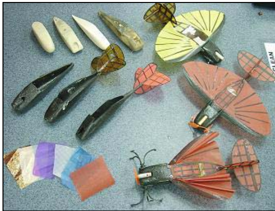
Fig. 6: Three completed vehicles are shown with a series of fuselage tools and an array of investigated wing fabrics.
