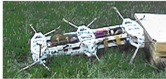
Figure 2. Whegs I uses three spoke whegs. A three-spoke wheg can reach the top of a barrier that is higher than the length of a spoke.
