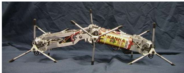
Figure 7. Whegs II can flex its body.
