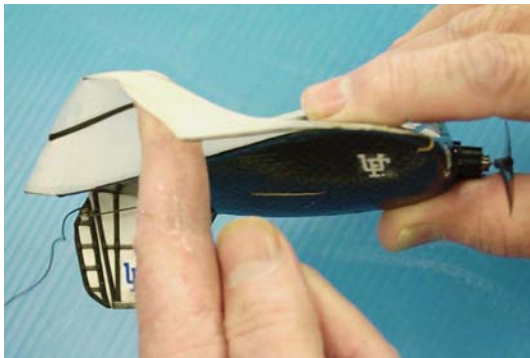
Fig. 2: Demonstrating the flexibility of the wing on the UF-MAV
