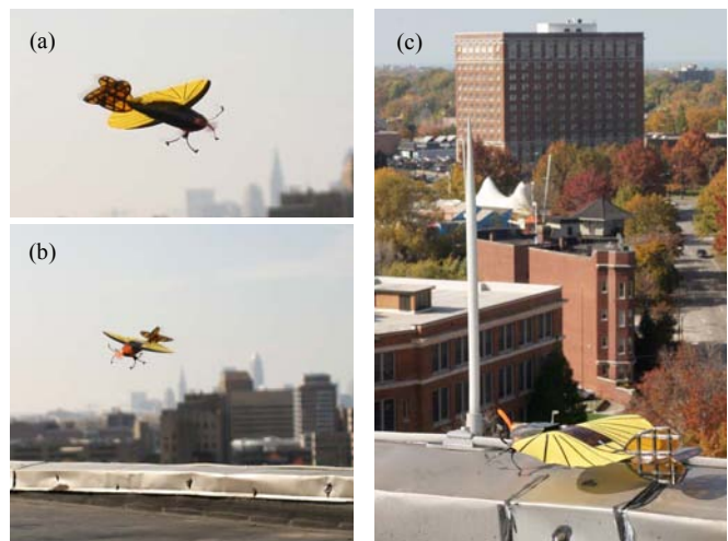
Fig. 1: In the proposed mission, MMALV must (a) fly up to 1.6km from the launch point to the target zone, (b) land on a rooftop within the target zone, and (c) walk to the edge of the building to survey the neighboring area.
